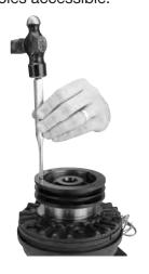
Note: For high cycle rate applications with potential pulley misalignment, apply Loctite to the I.D. of the pulley to eliminate the possibility of keyway wear.
