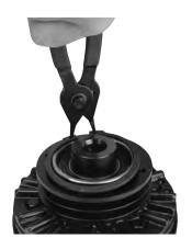
ACAUTION When installing this or other retaining rings, be sure to hold the ring with one hand so it will not spring away should the pliers lose their grip on the ring. Always wear safety glasses when installing or removing retaining rings.
