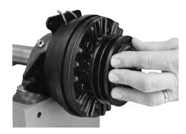
7. Tighten the hub setscrews into the shaft to the appropriate torque for your size unit:
